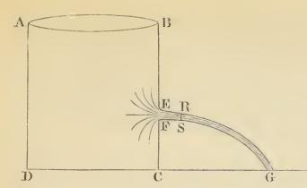
in a very thin plate of sheet tin. And conceive that the water converges towards the hole from all parts of the vessel & passes through the hole with
